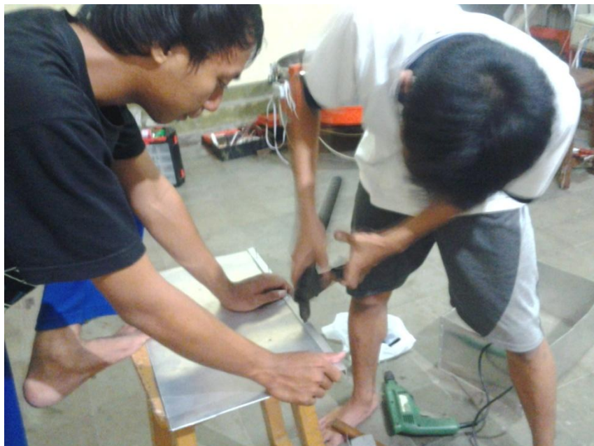
Gambar 5. Proses Merivet Plat
