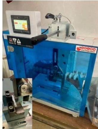
Gambar 2. 3 Uji Impak Charpy (Tunçel, 2024)
