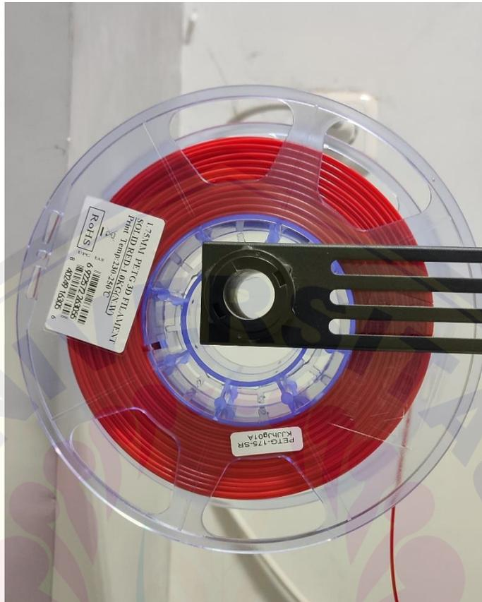
Gambar A.1 Filamen PETG (*Polyethylene Terephthalate Glycol*) Solid Red
