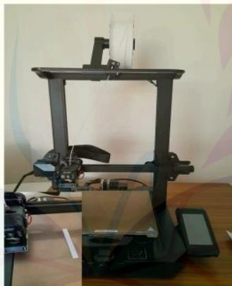
Gambar 2. 2 Mesin 3D Print FDM (Tunçel, 2024)
