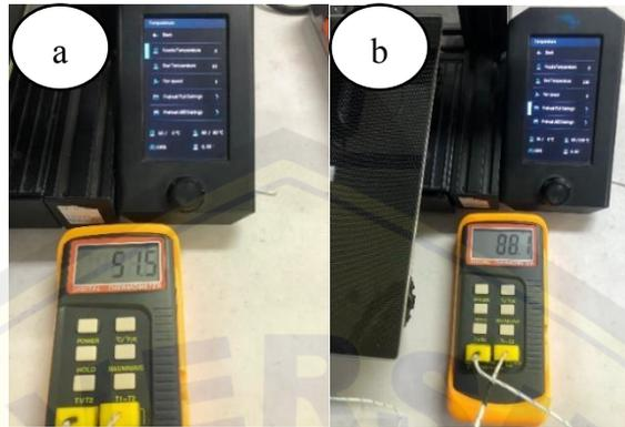
Gambar 4. 2 Validasi (a) suhu *bed temperature* dan (b) suhu nozzle
