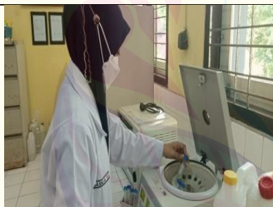
Pengujian water holding capacity
