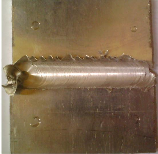
Lampiran A3. Hasil Pengelasan *Friction Stir Welding*
