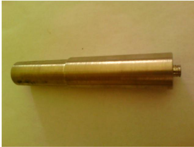
Lampiran A1. Tool Friction Stir Welding
