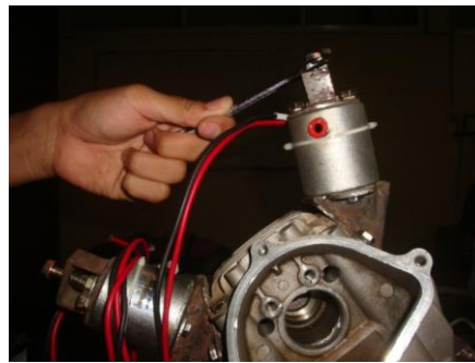
Gambar 4.9 Proses Penahan Poros Solenoid ( start )
