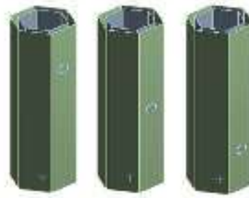
Figure 2. Distance position holes of multi-cell hexagonal crash box
