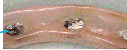
Figure 4: Magnet corrosion on a denture base.
