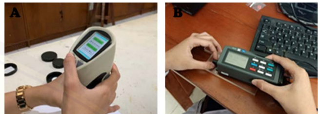
Figure 3. A. Acrylic plate color stability test, B. Acrylic plate surface roughness test.
