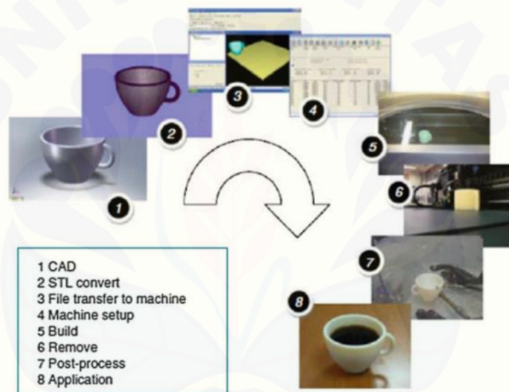
Gambar 2.3 Langkah-langkah pengoperasian 3D printing (Gibson dkk., 2015)
