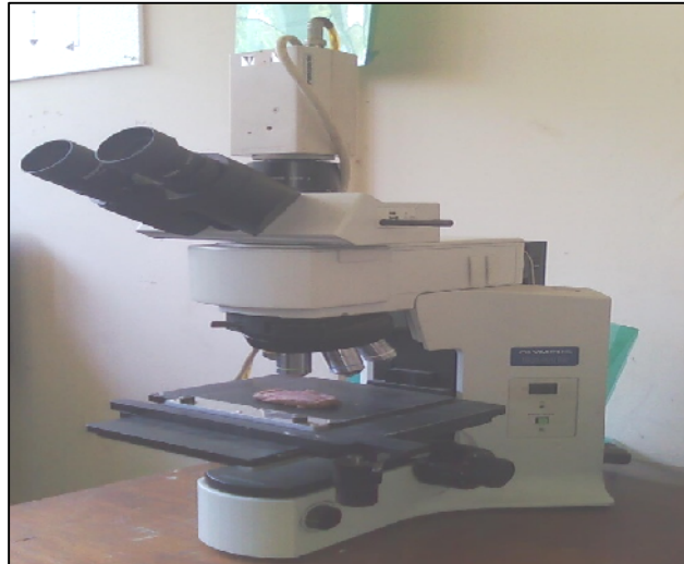
Gambar 3. Microscope Olympus dilengkapi alat uji kekerasan microhardness
