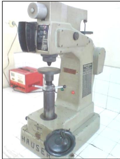
Gambar 3.4 Mesin Uji Electric Brinell Hardness Tester Hauser Henry S A
