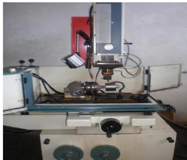
Gambar E.2 Mesin EDM *Die Sinking*
