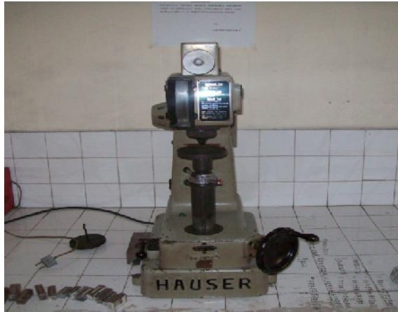
Gambar E.7 Mesin Uji Electric Brinell Hardness Tester Hauser Henry S A
