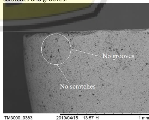
Figure 7. SEM image tool surface before marble rock machining
