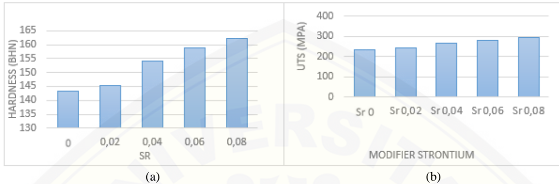
Figure-3. (a) Hardness value of Al-Si-Mg alloys with the addition of strontium modifiers, (b) Value of the tensile strength of Al-Si-Mg alloys with the addition of strontium modifiers.
