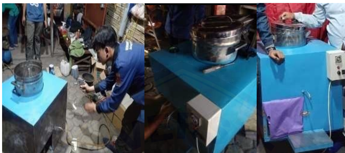
Figure 3. Semi-Automatic Honey Filter Machine
