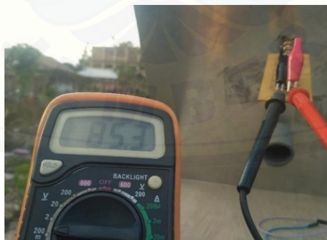
Figure 12. Testing of Energy Harvesting Rectenna
