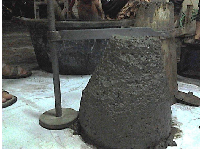
Gambar E.7 Proses Uji Slump Beton Normal
