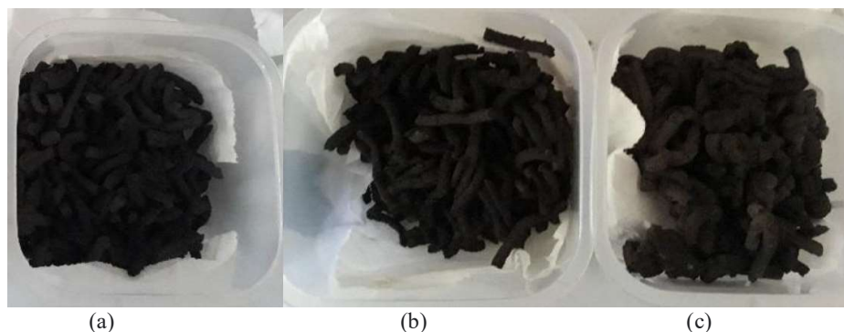
Figure 1. Combined biopellet fertilizer of biochar: chicken manure: fish waste a) 70:15:15; b) 50:25:25; and c) 20:40:40.
