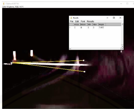
Gambar B.10 Pengujian Angle of Spray B 0 T 70°C Percobaan 1
