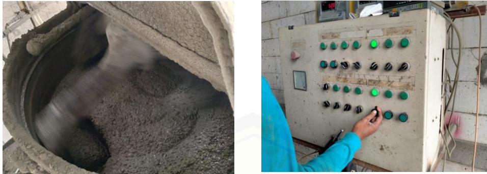
Gambar 2.6 Gambar Sistem Mixer Mesin Batching Plant
