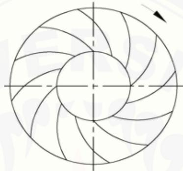
Gambar 2.3 *Blower sentrifugal Tipe Backward Curved Blade*
