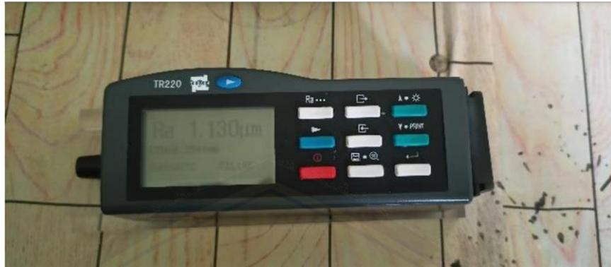
Gambar 3. Mesin Uji Kekasaran Permukaan (roughness tester TR220)
