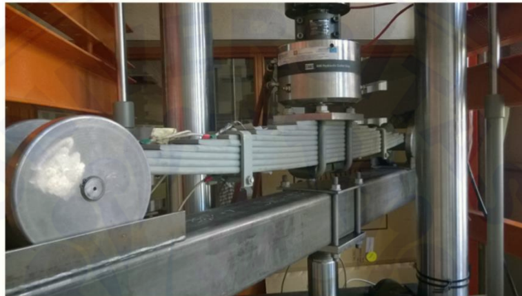
Gambar 2.4 Semi-Elliptical Spring Test (Mairusz, 2018)
