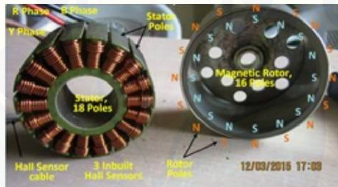
Gambar 2.5 Konstruksi motor Brushless Direct Current
