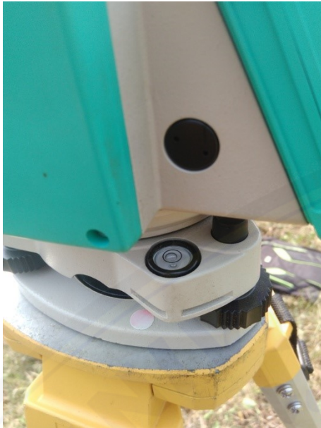
Gambar 26 Proses Centering Nivo Bulat
