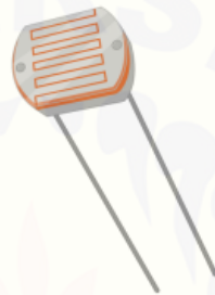
Gambar 2.7 LDR ( Light Dependent Resistor ) (Suhaeb et al. , 2017).
