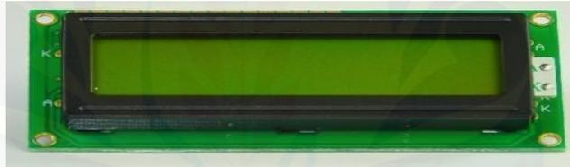
Gambar 2.7 LCD 2X16
