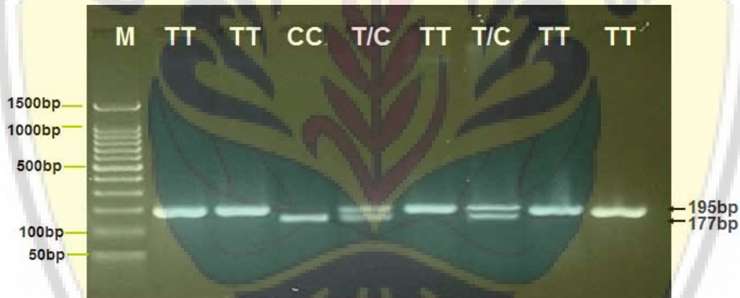
Figure (1): Agarose gel electrophoresis image that show the RFLP-PCR product analysis of IL-4 gene polymorphism (rs2243250) (T/C) by using Ava II restriction enzyme in 2% agarose. Where M: marker (1500-500bp), lane (TT) wild type homozygote that showed undigested by restriction enzyme as 195bp. Lane (T/C) heterozygote, the product digested by restriction enzyme into 195bp, 177bp and invisible 18bp. Lane (CC) mutant type homozygote, the product digested by restriction enzyme into 177bp and invisible 18bp bands
