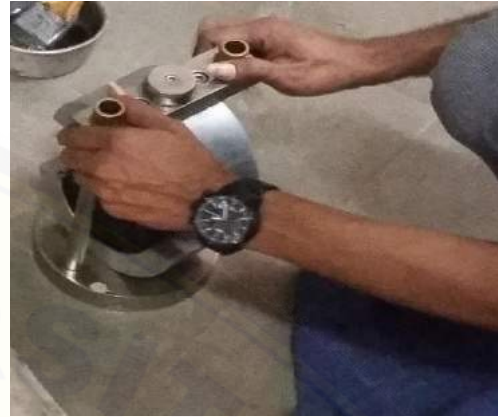
Gambar 19 Proses Pengujian Marshall.
