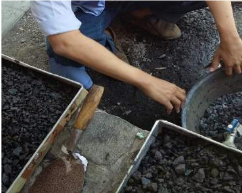
Gambar 1 Proses Pencucian Agregat
