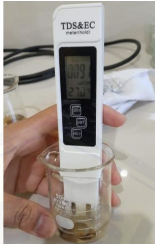
Gambar 3.6 Mediatech 1900131 TDS EC Meter (Sumber: dokumen pribadi)
