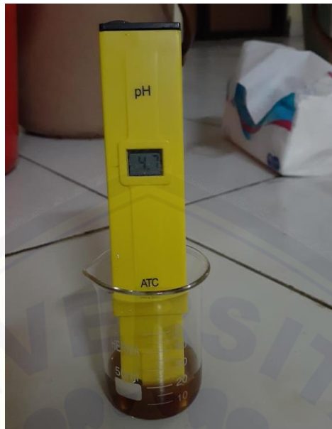
Gambar 3. Pengukuran nilai pH green coffee robusta
