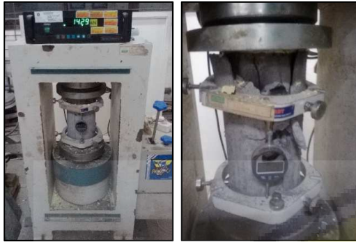
Fig. 1 The compressive strength test setting of the concrete cylinder.
