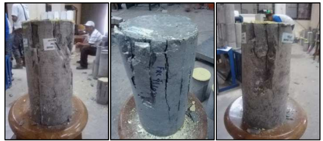
Fig. 2 The crack pattern of φ15 cm x 30 cm cylinder specimen
