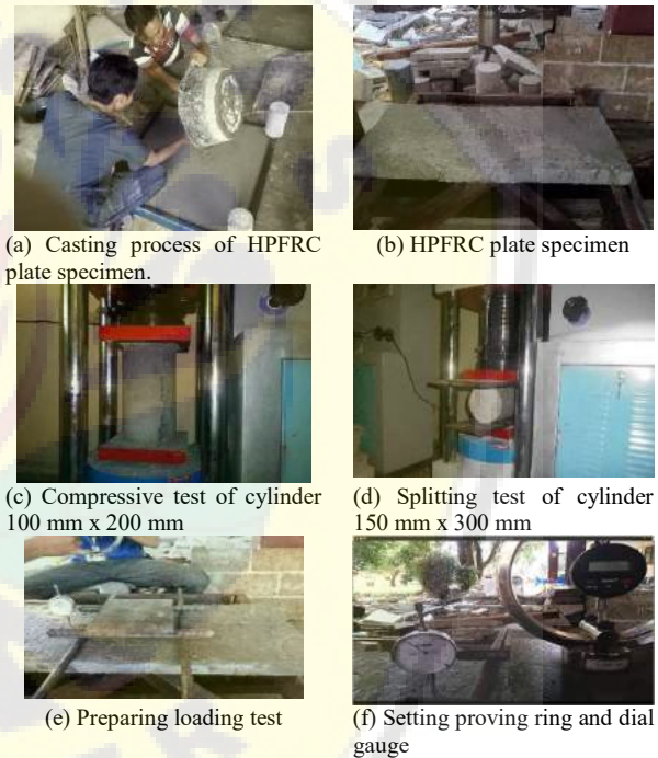
Fig. 4 Preparing and testing HPFRC cylinder and plates
