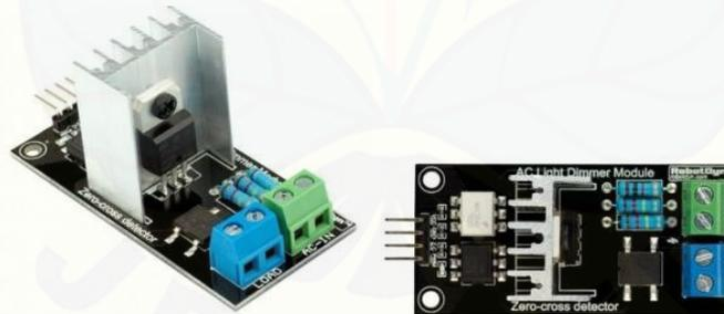
Gambar 2.2 AC Light Dimmer Module
