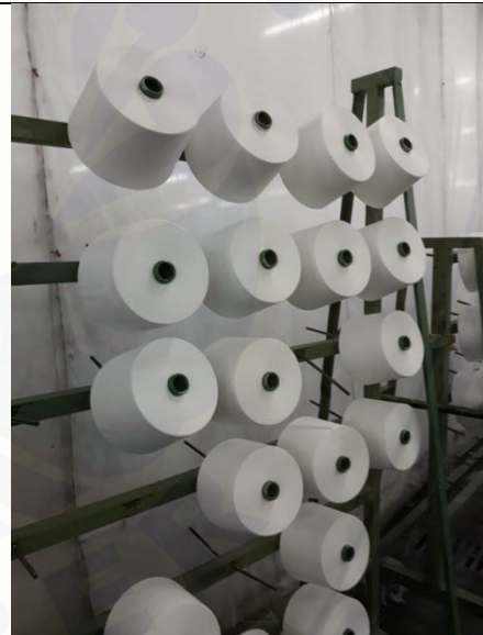
Gambar 12. Hasil proses winding (gulungan benang besar)
