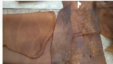
Gambar 18. Proses sortasi Ribbed Smoke Sheet (RSS)
