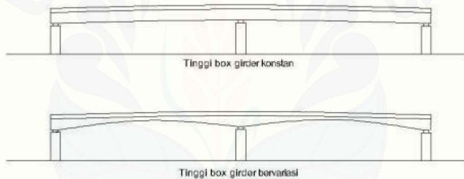
Gambar 2.12 Macam-macam tinggi box girder
