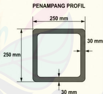
Gambar 4.2 Penampang Profil HSS Square
