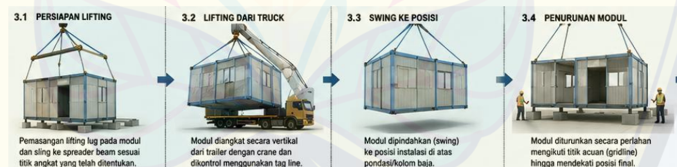
Gambar 4.6 Alur Lifting Modular
