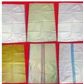
Gambar 2.4 Karung plastik berbahan polypropylene homopolymer (Ali, 2013)
