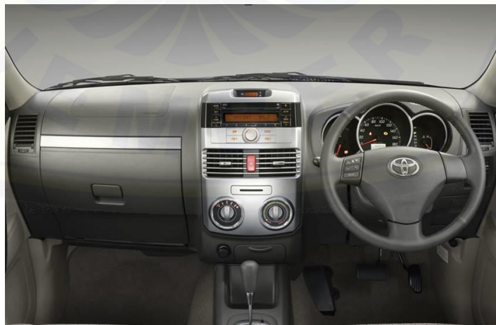
Gambar 2.6 Dashboard mobil berbahan polypropylene impact copolymer (Ali, 2013)
