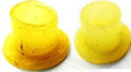
Gambar 2.14 Cacat shrinkage (Mawardi dkk, 2015)
