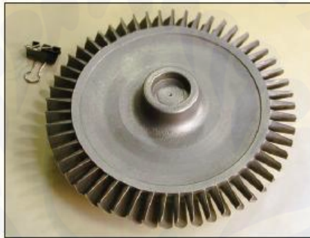
Gambar 2.9 Turbin Disk contoh produk hasil MIM (Virdhian, 2014)
