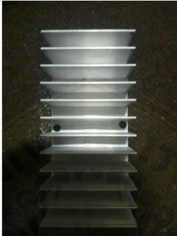
Gambar H. 3 Variasi luasan *heatsink* 72 cm<sup>2</sup>
