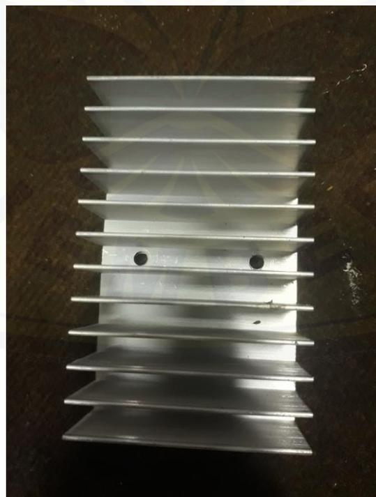
Gambar H. 2 Variasi luasan *heatsink* 96 cm<sup>2</sup>
