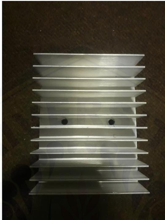
Gambar H. 1 Variasi luasan *heatsink* 120 cm<sup>2</sup>
