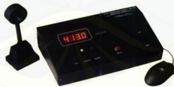
Gambar 2.1 Reaction Timer Center L-77
