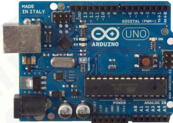
Gambar 2.3 Board Arduino Uno
