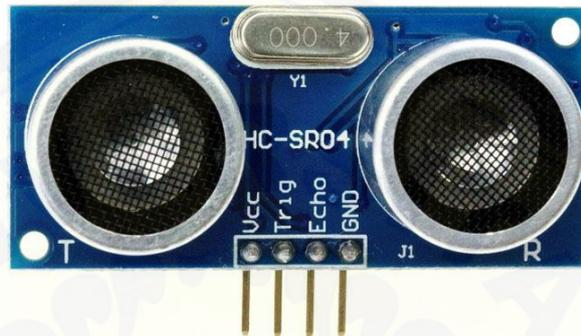
Gambar 2.6 Sensor Ultrasonik HC-SR04
