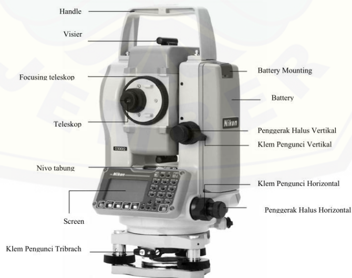
Gambar 2.7 Total Station (Nikon DTM 322 ). (Sumber :Manual Praktis Nikon DTM 322 )
