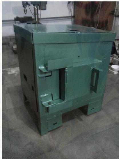
Gambar D.14 Rangka *Muffle Furnace*
