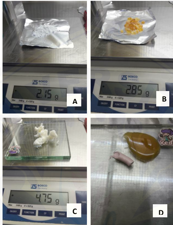
A. Zinc Oxide , B. Rosin , C. Hydrogenated fat , D. Periodontal dressing Coe-pak .
