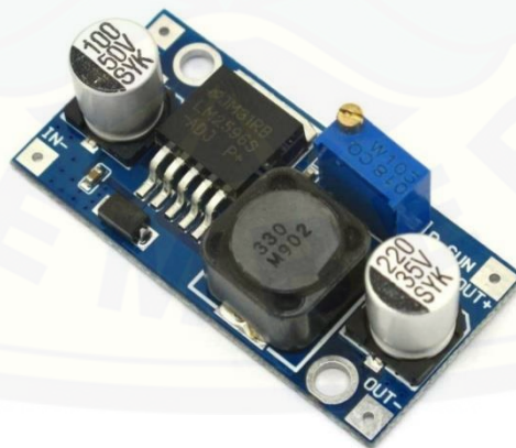
Gambar 2.5 LM2596 DC-DC Step Down
