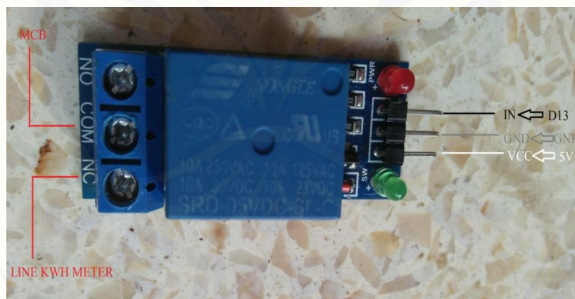
Gambar 3.5 Relay 5V 1 Channel output 250V AC 30V DC 10A
