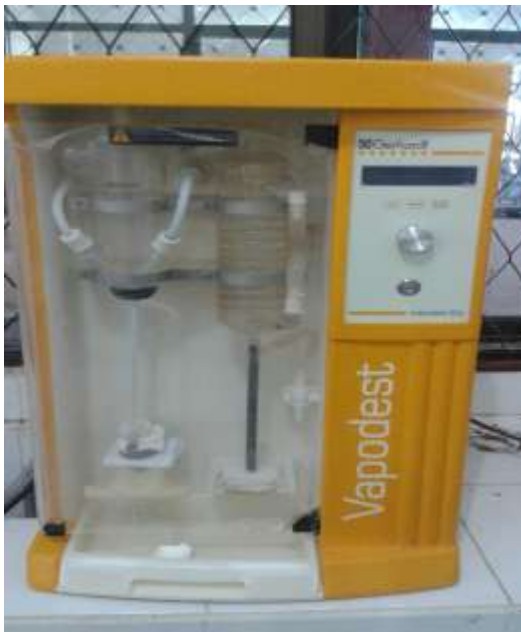
Gambar 9. Alat Destilasi Uji Protein
