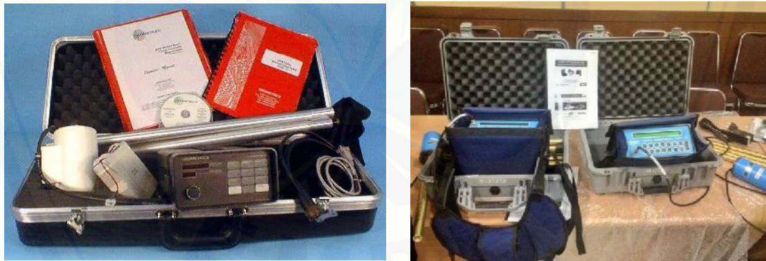
Gambar 2.5 Proton Precession Magnetometer (Sumber: http://georesults.com.au/product/geometrics-g-857-proton-magnetometer )
