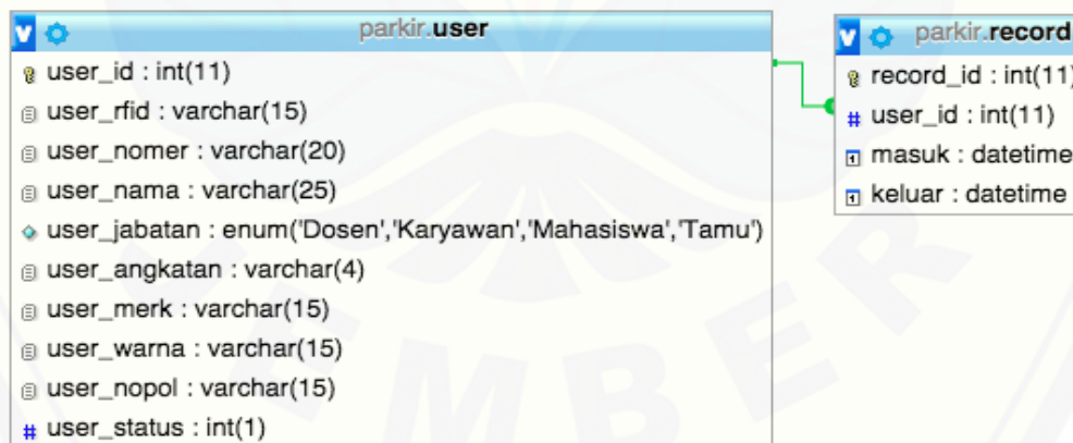
Gambar 4.8 Entity Relationship Diagram Sitem Parkiran Kendaraan Bermotor roda dua
