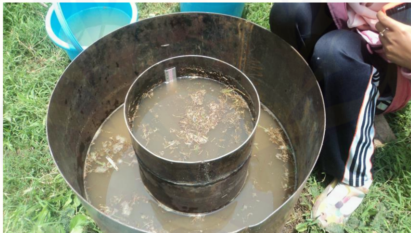
Gambar 4.1 Double Ring Infiltrometer
