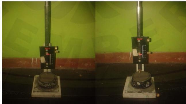
**Gambar 10.** Pengujian *Setting Time*
