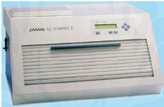
Gambar 2.7 Densitometer CAMAG (Satiadarma et al. , 2004)
